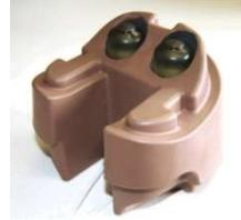
For impact testing, the sensors are inserted vertically by pair in the abdomen.
