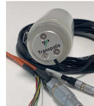
The APTS are mounted inside special Q dummy abdomen. These abdomen assemblies are designed by Humanetics Innovation Solutions or Cell Bond featuring two blind holes parallel to the lumbar spine.
