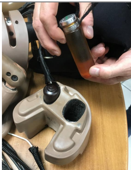
Preparation of APTS cable routing inside Q6 abdomen
