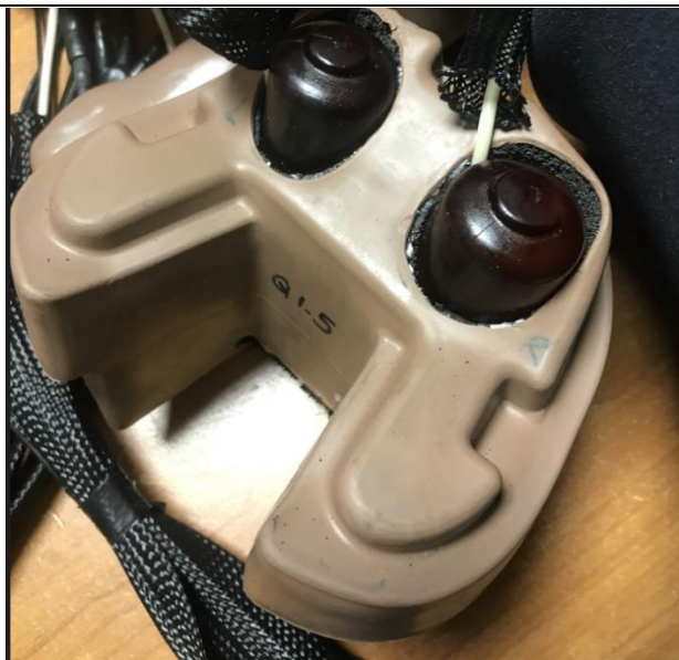
View of APTS pair inside abdomen with cable output along the sensor (not recommended)
