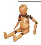
Since 2016, Transpolis has been manufacturing Abdominal Pressure Twin Sensors (patented by Gustave Eiffel University) for the Q-series infant to child dummies used for crash tests (front and side impact testing). APTS sensors are an essential tool for in-depth assessment of child restraint systems. This is a unique sensor to evaluate abdominal injury risk and submarining for occupant safety prediction.
