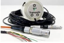
The ability of the restraint system to meet injury regulatory criteria is assessed by recording the pressure inside the abdomen during the crash impact. The sensors are inserted vertically by pair in the abdomen. They are available in 3 sizes: 30, 40 and 50 mm.
