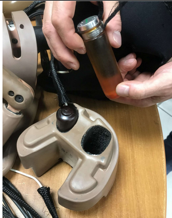
Preparation of APTS cable routing inside Q3 abdomen
